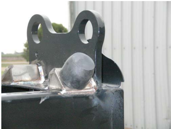
After weldment and painting are complete screw in rubber bumper as shown.
