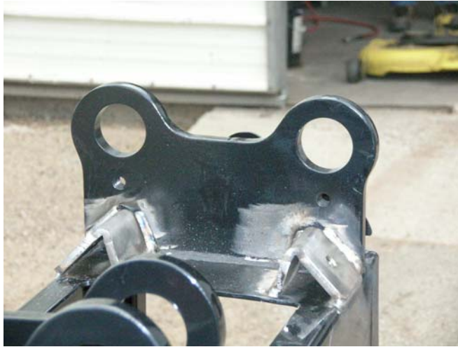
Mount brackets flush with channel.
